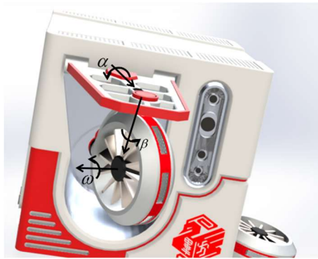
Fig. 17 Structure of variable-speed double-gimbal fan
